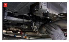
The valve motors on the original system are required when fitting the Scorpion system.
