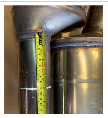
We recommend removing the original system from the flange joint before cutting.
